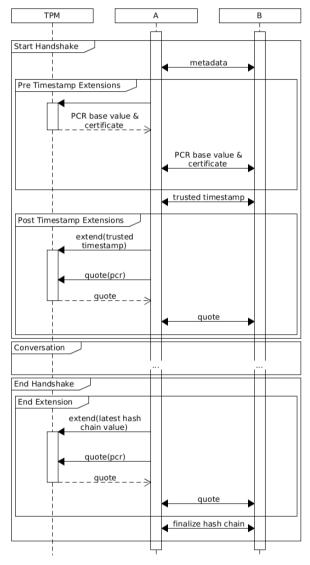
Figure 3. TPM integration via protocol extension
