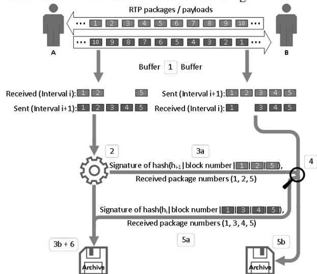
Figure 1. Flow diagram of communication between parties A and B
