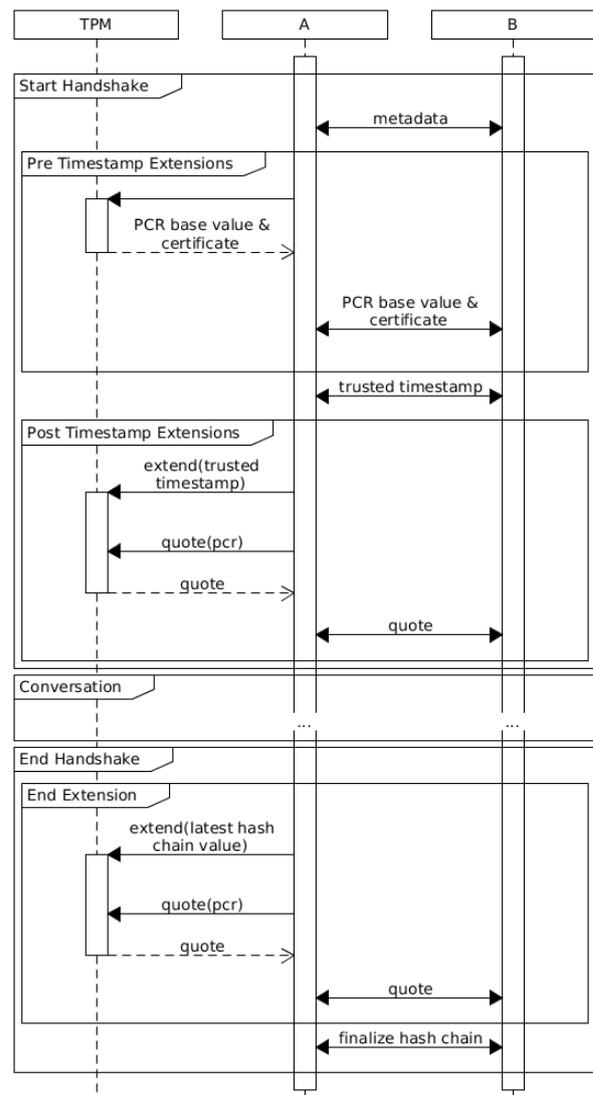
Figure 3. TPM integration via protocol extension
